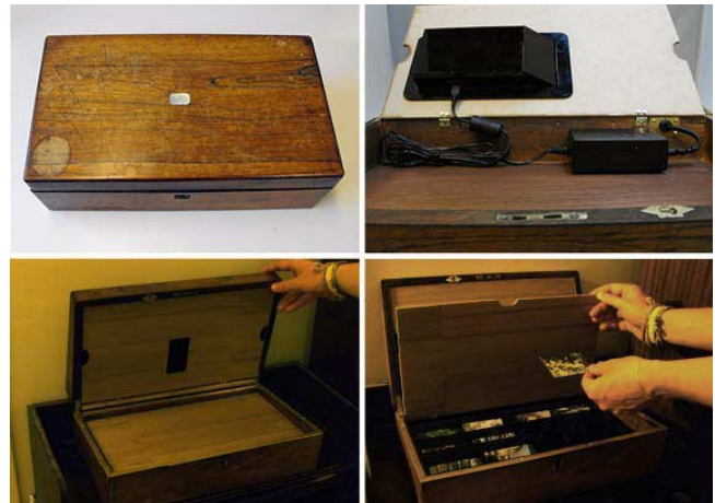
Figure 1. Clockwise from top left: The writing box before it was augmented; Upper panel (open) where printer components are hidden; Photobox can be opened to see if a photo has been printed; Bottom panel for photo organization and storage.
